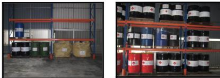
Figure 5: Crate storage of scheduled wastes
